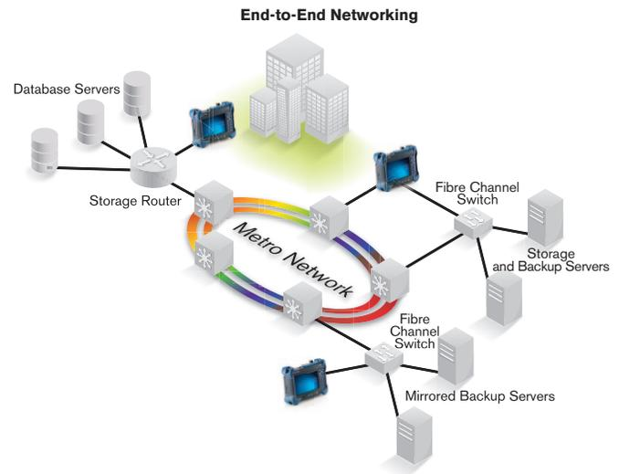
*Thanks to end-to-end network testing capabilities, EXFO's FTB-700G Series enables fast deployment and configuration of Fibre Channel networks. Communication between the transport network, interconnection devices and end nodes can be validated with features such as BER testing, latency measurement, buffer-to-buffer credit estimation and port login capabilities.*
